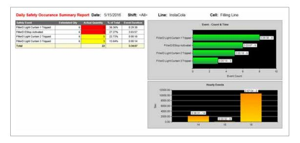
Use frequency that is significantly higher than anticipated could be the result of a product or process change that needs to be addressed. And use frequency that is lower than expected could indicate that a safeguard is being defeated and needs to be re-evaluated.
