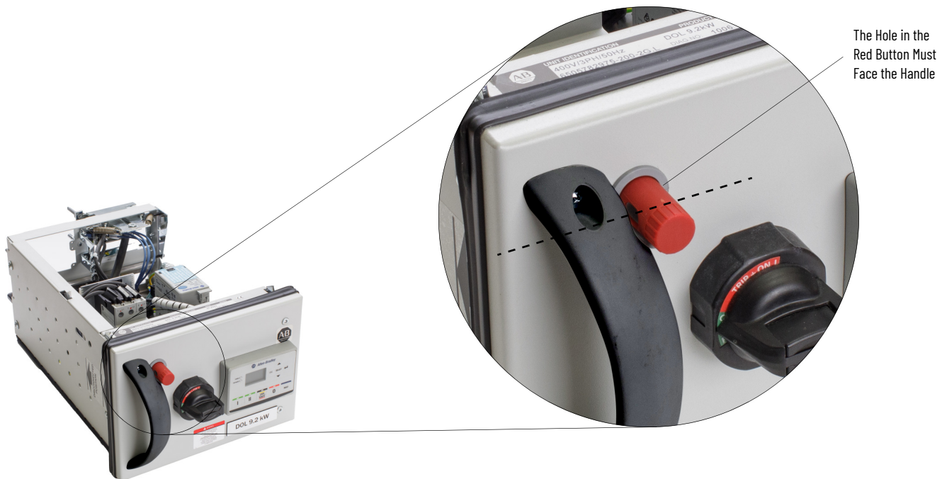
Figure 42 - Withdrawable Unit Button Alignment
