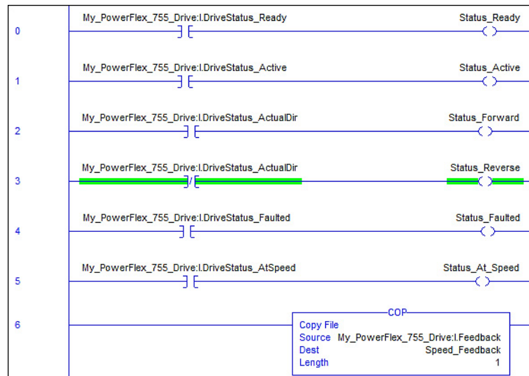
Figure 14 - ControlLogix Controller Example Ladder Logic Program Using a Drive Add-on Profile for Logic Command/Reference
