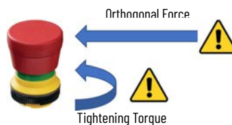
Figure 34 - Proper Use and Mechanical Limits of Actuator
