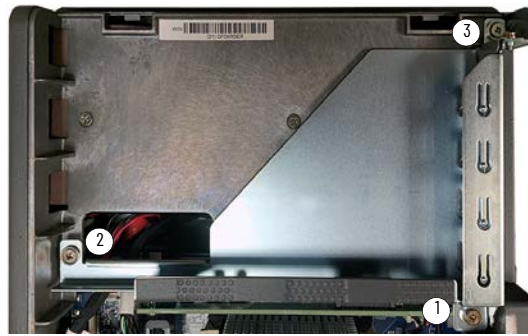
Figure 13 - Add-in Card Tray – Screw Locations and Tightening Sequence
