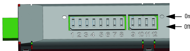
Figure 32 - DIP Switch Location at Receiver Plug-in
