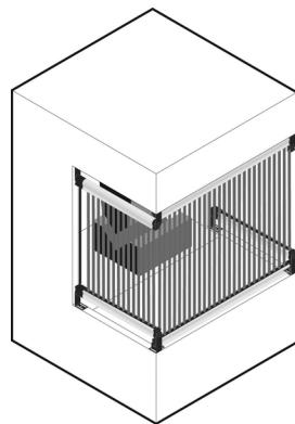
Provides 3-sided machine guarding without the use of corner mirrors.
