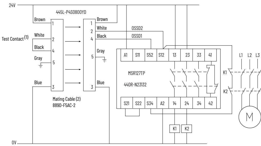
(1) Jumper required for normal operation.
