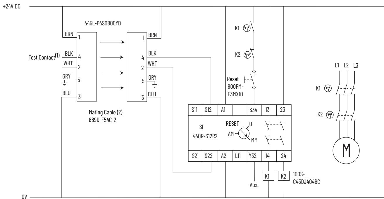
(1) Jumper required for normal operation.
