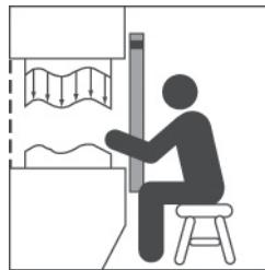
Operators cannot reach hazardous machine parts without passing through the protective field.
