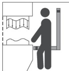
Operators must not step between protective field and hazardous machine parts (by-pass prevention).
