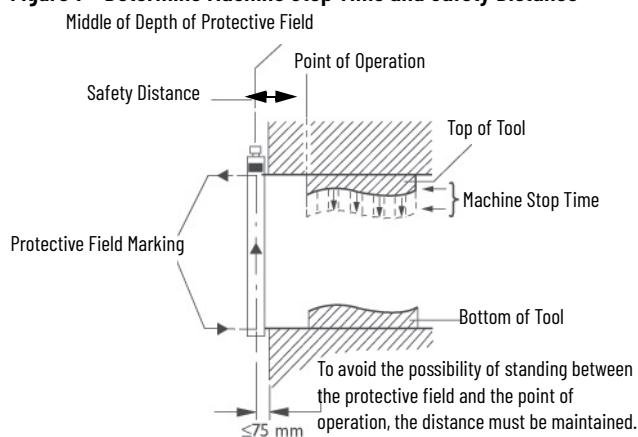
After the installation and alignment of the GuardShield Safe 4 safety light curtain, the protection field must be tested with the test rod for the corresponding resolution [14 mm (0.55 in.) or 30 mm (1.18 in.)] according to [Figure 8 on page 24](#).
