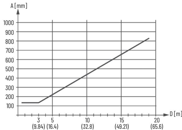
The effective aperture angle for the GuardShield Safe 4 safety light curtain system is  $\pm 2.5^\circ$  at a mounting distance of  $> 3.0$  m (9.8 ft). Calculate the minimum distance to reflective surfaces depending on the distance between the transmitter and the receiver, with an aperture angle of  $\pm 2.5^\circ$ . Alternatively, take the appropriate value from the [Table 1 on page 19](#).
