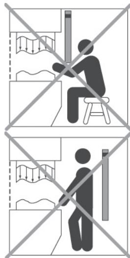
Operators can reach hazardous machine parts without passing through the protective field.
