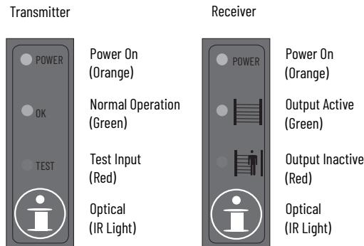
The status indicators on the transmitter and receiver indicate possible errors and operation status.
