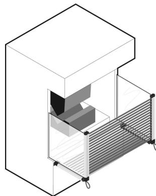
Offers protection when it is possible to stand between the vertical safety light curtain and the machine hazard.
