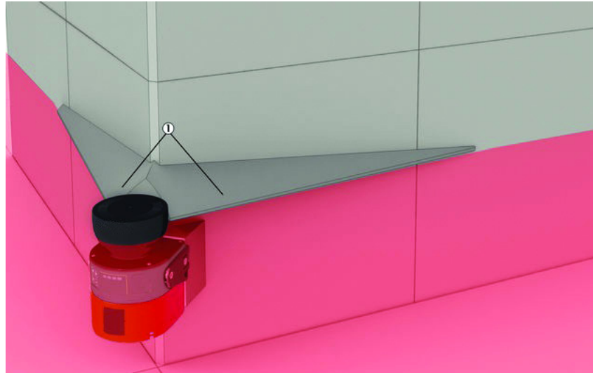
Figure 20 - Mounting with Deflector Plates (Example)
