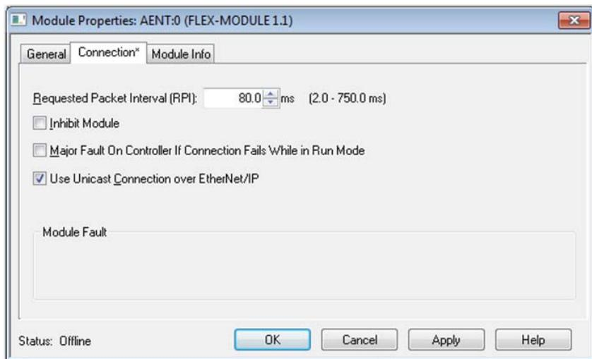
10. Set the RPI value to 80 ms and check Use Unicast Connection over EtherNet/IP™.
