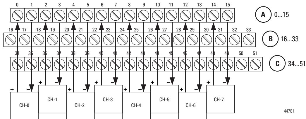
**NOTE:** Loop power is not provided for the inputs. Each input requires an external power source, as illustrated in the following diagram.
