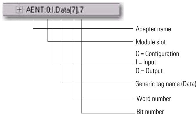
To be able to use the generic tags, you can consult the tables in the following section for designated tag names for each bit. For example, the following tag name refers to the Fault Enable configuration bit for Channel 0.
