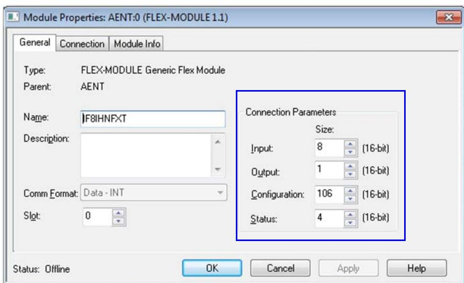
The Size box determines how large the connections are between the owner-controller and the I/O module. Connections are sent in sizes matching the selected communication format data type.
