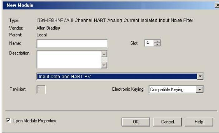
2. Click Open Module Properties. The Module Properties dialog appears and has the following tabs available for configuration.
