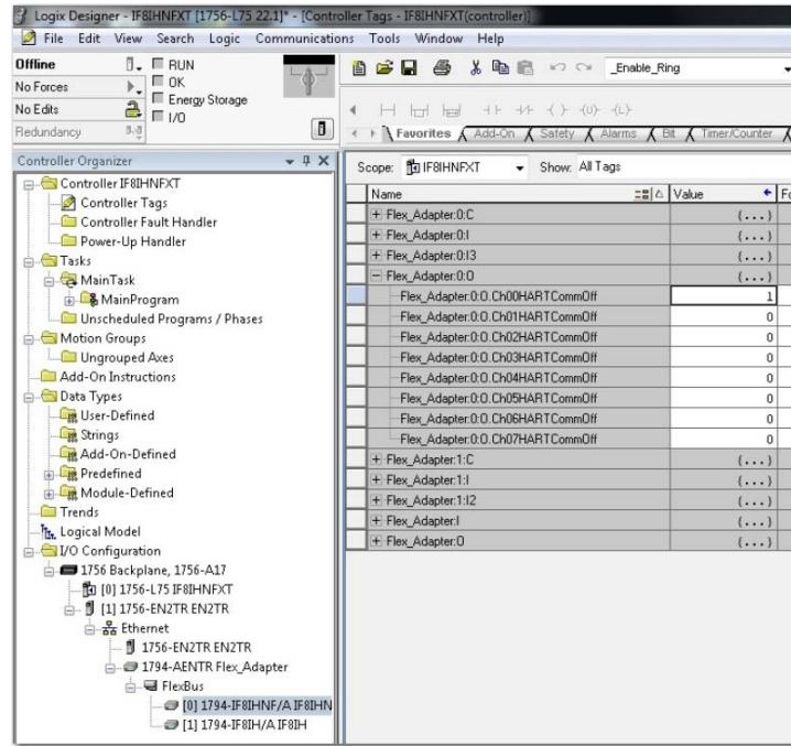
The HART OFF dynamic control output bit, along with the HART Disable configuration bit, determines if HART communication is enabled on a Channel. The HART Disable (DHn) configuration bit has priority and disables all HART communication on a channel at all times even when the HART OFF output bit is False(0). If the HART Disable configuration bit is False(0), then the HART OFF output control bit can be used to turn HART off and on dynamically at any time.
