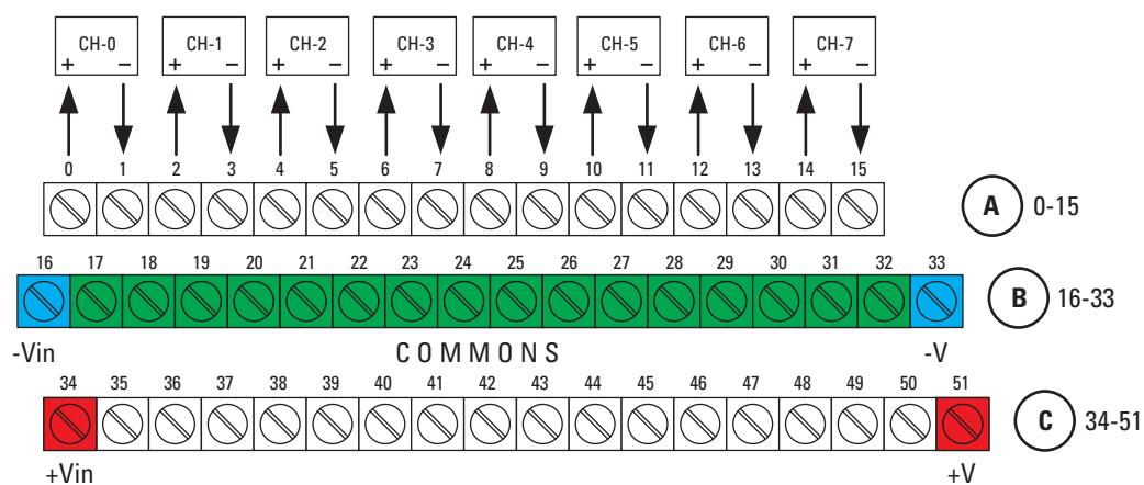
Connect an external 24V DC power supply to terminals 34 (V+) and 16 (V-) observing polarities indicated. Terminals 17...33 are internally shorted to terminal 16. Terminal 51 is internally shorted to terminal 34. Use the DC output terminals only for low-power modules, following FLEX I/O power connection guidelines.
