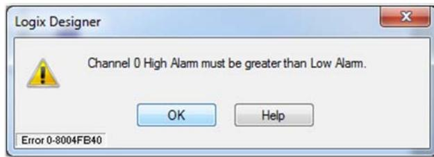
3. Low Alarm must be greater than Low Low Alarm. If not met, the following error message is displayed.
