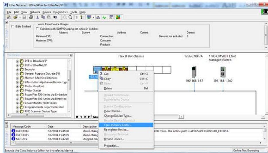
3. Through the Class Instance Editor window, send Get Device Information Block 1 message to channel 1 of 1794-IF8IHNFXT module in Slot 0. To do this:
