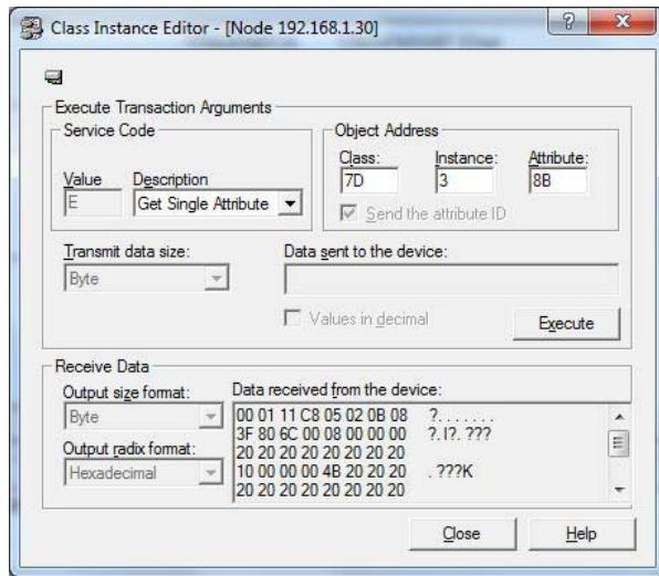
Note that there are 48 bytes of data returned from the module. See the following tables to understand message reply and request message structure from the device:
