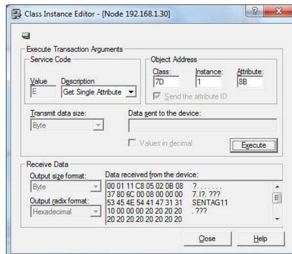
Note that there are 56 bytes of data returned from the 1794-IF8IHNFXT device as indicated in the Receive Data section of the dialog box.
