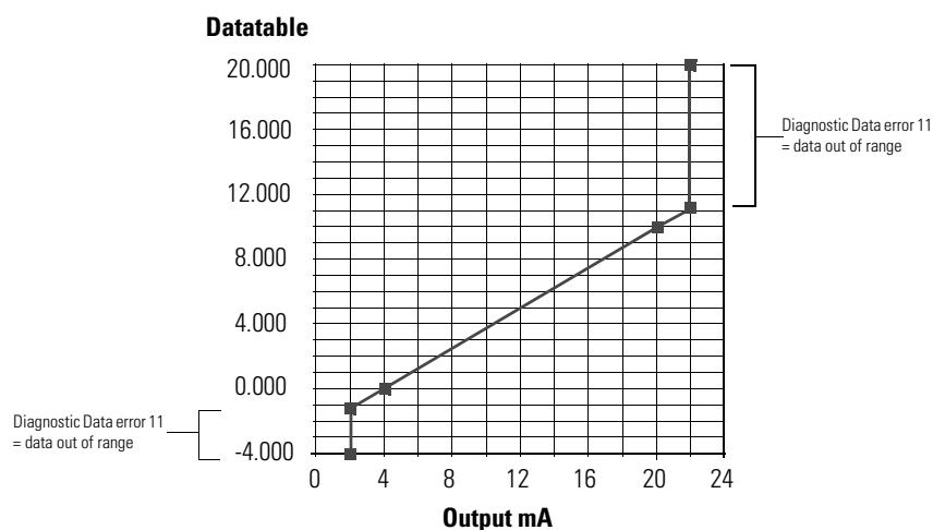
For data format tables and a more detailed description of the data formats for the 1794-OF8IH module, see [Data Format \(Configuration Words 2, 3 – bits 0...3, 4...7, 8...10, 12...15\) on page 76](#).
