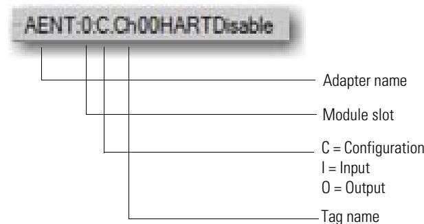
2. To enable HART on channel 1, set the value of the Ch0HARTDisable tag to 0. The default value of 0 indicates that HART is enabled by default in the channels.
