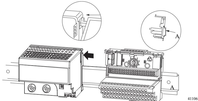
5. Slide the terminal base over tight against the adapter (or proceeding terminal base). Make sure the hook on the terminal base slides under the edge of the adapter (or proceeding terminal base) and the Flexbus connector is fully retracted.
