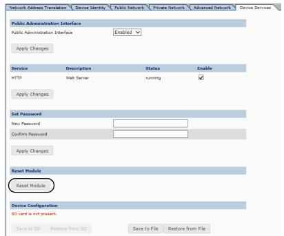
20. At the device reset warning window, click Reset Module.
