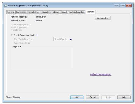
Click Advanced to display the Advanced Network Configuration dialog box. You can configure supervisor mode and ring parameters in the dialog box. Click Set to apply any changes.
