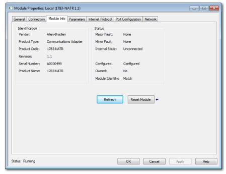
Module faults display in the Status area of the Module Info tab. Minor faults are recoverable and major faults are nonrecoverable. The module becomes uncommunicative with a major fault. In the following figure, a change in DIP switch configuration after powerup caused the minor fault. The minor fault can be recovered by returning the DIP switches to the correct configuration.
