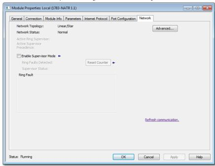
When Enable Supervisor Mode is selected, ring faults display in the Ring Fault area of the Network tab.
