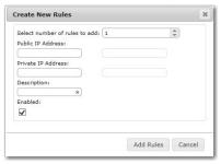
**2.** Configure the dialog box as necessary for your application and click Add Rules. Each additional IP address automatically increments by one.
