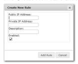
2. Configure the dialog box as necessary for your application and click Add Rule. The private IP address is the IP address that is configured on the device on the private network. The public IP address is the translated address that devices on the public network use to communicate with the device on the private network.
