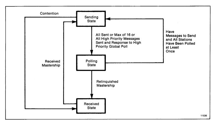
Figure 2.5 — State Transition at Master Station
