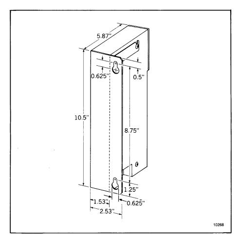
Figure 3.5 — Mounting Dimensions for 1771-KF Module
