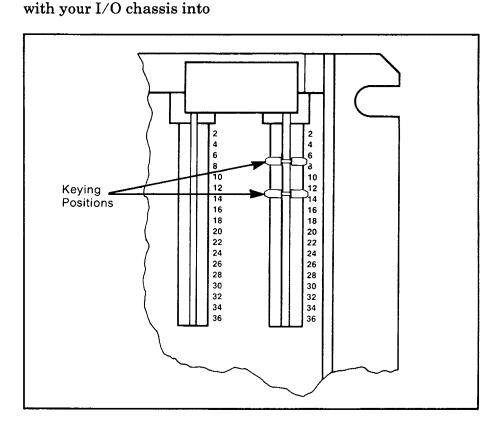
You can change the positions of keying bands if subsequent system design requires the insertion of a different type of module in this slot.
