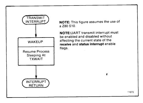
Figure B.17 — TRANSMIT INTERRUPT Subroutine
