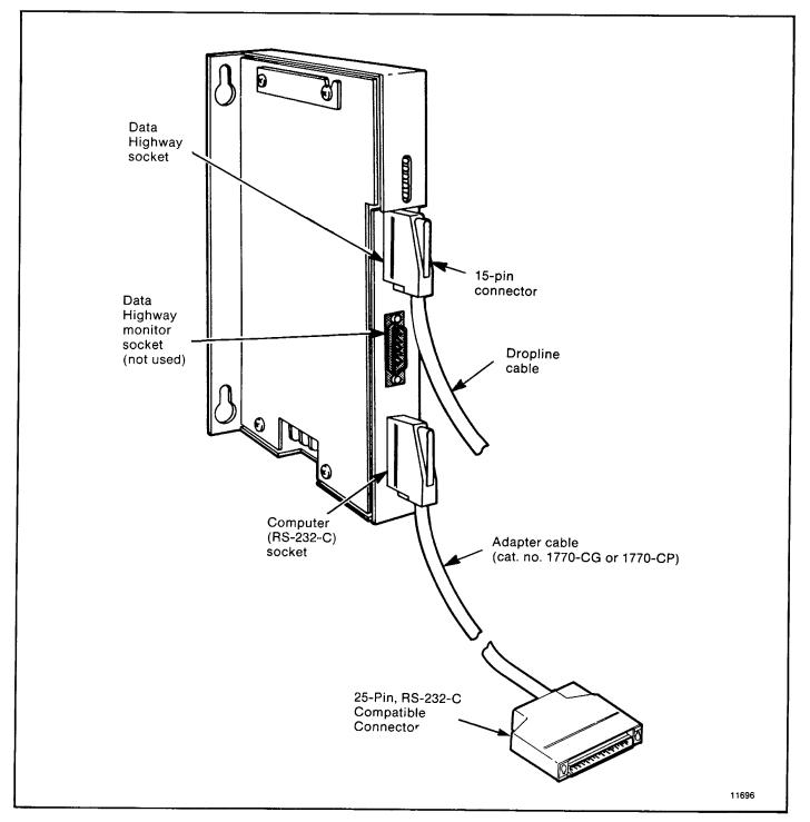
Figure 3.8 — KE/KF Module Connectors
