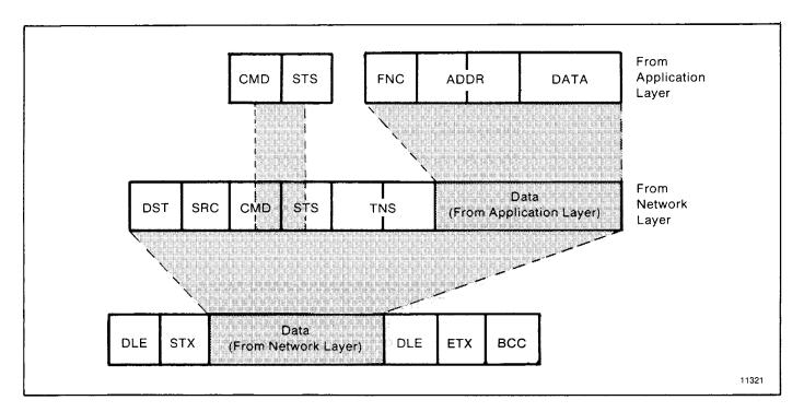
Figure 4.1 — Link Packet Format for Full-Duplex Protocol
