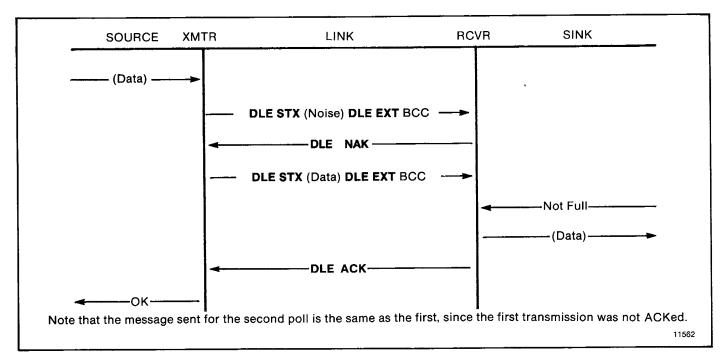
Figure 4.10 — Message Transfer with NAK
