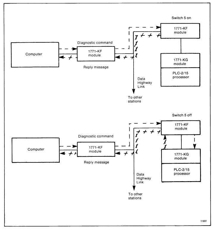
Figure 3.3 — Effect of Switch 5 on Diagnostic Commands
