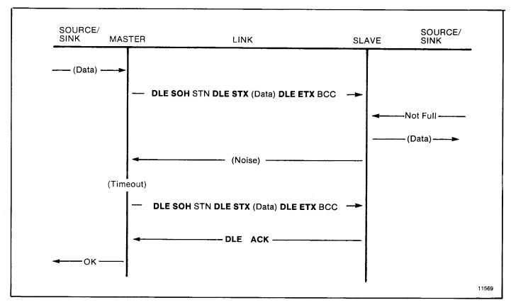
Figure 4.19 — Message Transfer with ACK Destroyed
