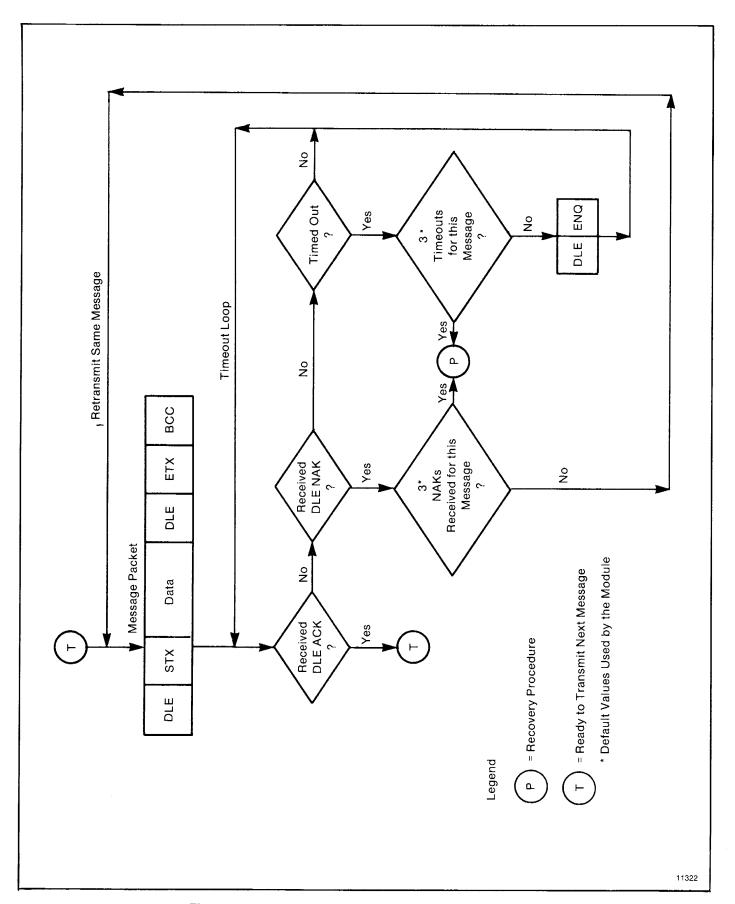
Figure 4.7 — Software Logic for Implementing Transmitter
