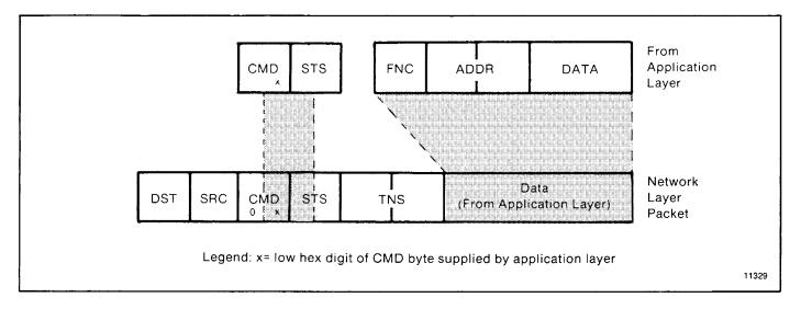
Figure 5.2 — Command Message Packet Format
