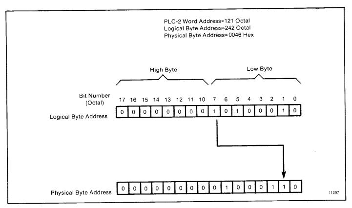
Figure 6.8 — Converting PLC-2 Logical to Physical Address
