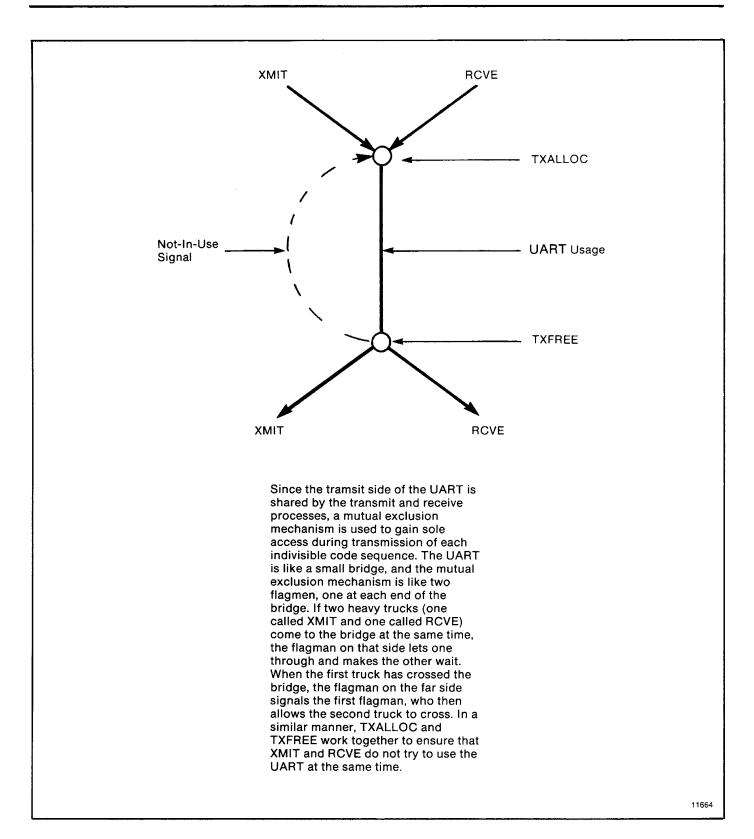
Figure B.10 — Sharing the Transmit Side of the UART
