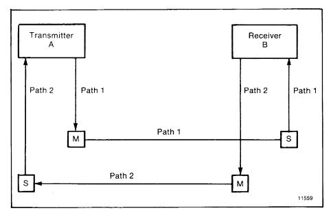
Figure 4.5 — Message Transmission from A to B
