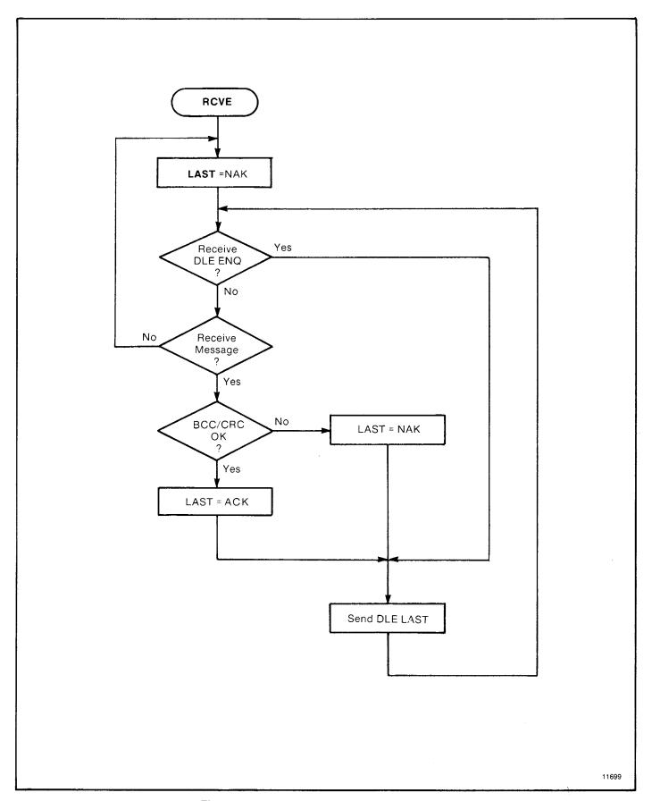
Figure 4.8 — Receiver for Full-Duplex Protocol
