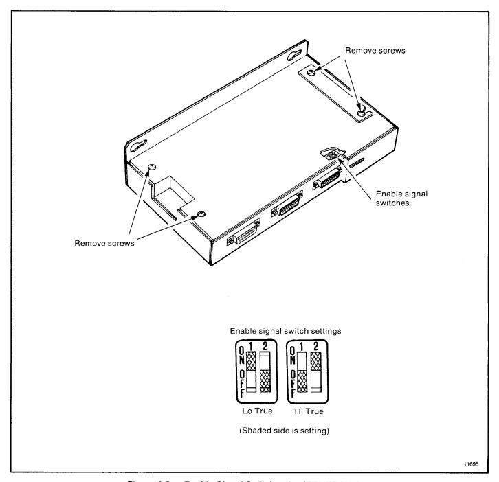
Figure 3.7 — Enable Signal Switches for 1771-KF Module
