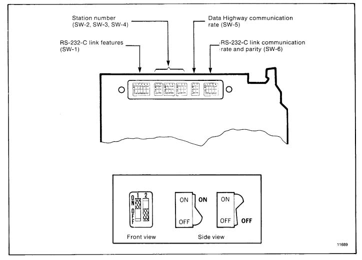
Figure 3.1 — Communication Option Switches
