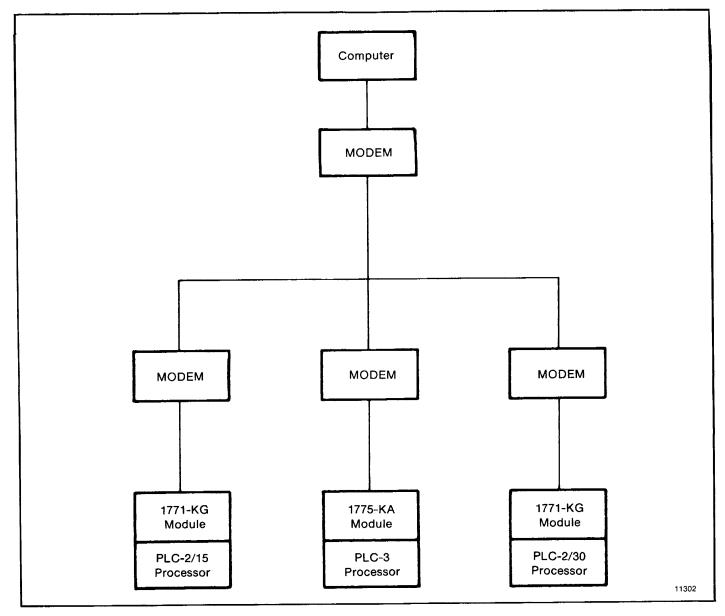
Figure 2.4 — Stand-Alone Multidrop Link to a Computer
