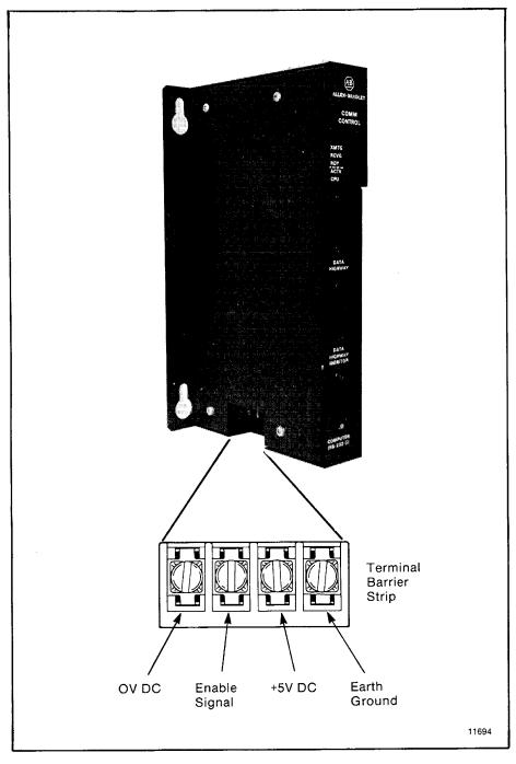
Figure 3.6 — Power Supply Connections for 1771-KF Module
