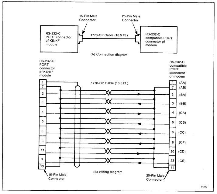
Figure 3.10 — Connection to a Modem
