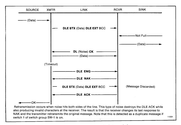
Figure 4.12 — Message Transfer with Retransmission
