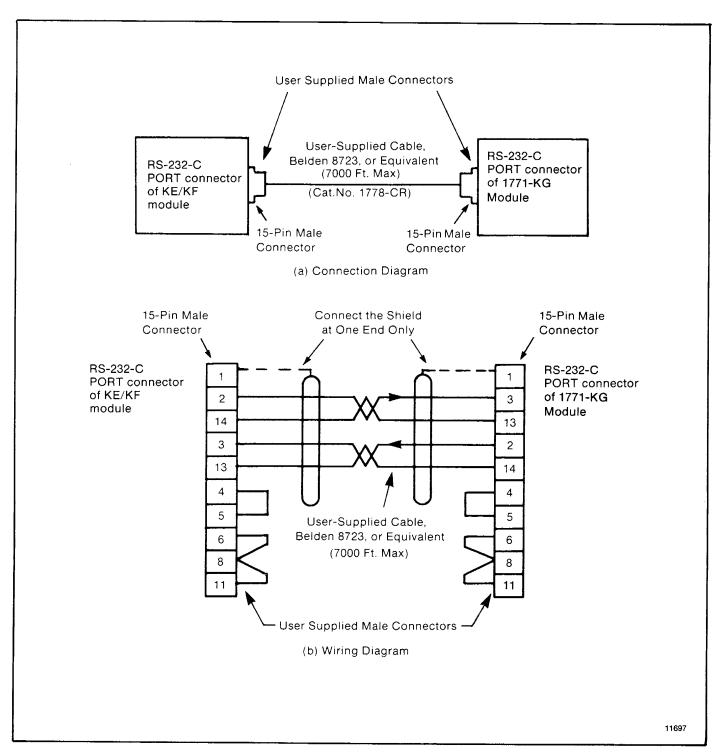
Figure 3.11 — Connection to 1771-KG Module
