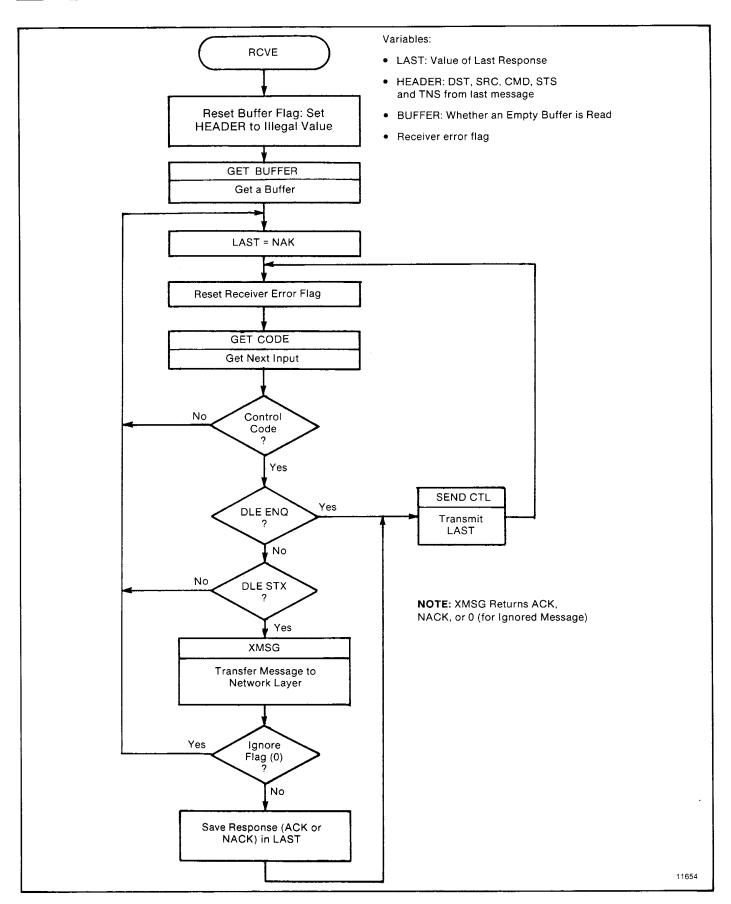
Figure B.24 — Receiver Routine for Full-Duplex Protocol
