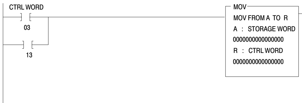
Figure A.17 Resetting the Control Word after a Block Transfer Error
