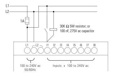
When using a 100 nF capacitor, the drop-off time of the input increases by 66.6 ms at 60 Hz (80 ms at 50 Hz). Also, a capacitor increases the amount of current seen by the input device. Do not use a bleeder capacitor in conjunction with reed switches.
