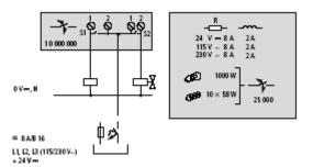
Unlike inputs, you can connect different phases to the outputs.
