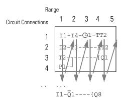
In the first three segments, Pico evaluates the contact fields in succession. As it does so, Pico also checks whether contacts are connected in parallel or in series and stores the switching states of all the contact fields.
