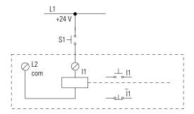
Connect devices such as buttons or switches to Pico input terminals.
