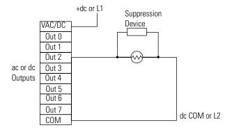
If the outputs are dc, we recommend that you use an 1N4004 diode for surge suppression, as shown below.
