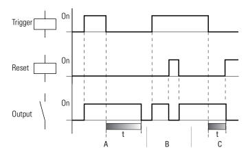
The trigger coil switches the contact. If the trigger coil (A) drops out, the setpoint time starts and resets the contact after the time has elapsed. The reset coil has priority over the trigger coil and always resets the relay contact (B, C). If the time is set to zero, the contact follows immediately after the trigger signal.
