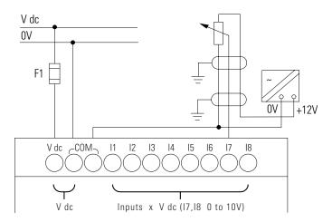
V dc = 12Vdc for 1760-L12DWD V dc = 24V dc for 1760-LxxBWB-xx
