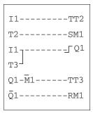
The enhanced Pico circuit diagram: after four hours, the continuous lighting is also switched off.
