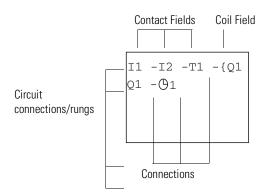
Connections are used to produce the electrical continuity between relay contacts and the coil. Connections can be created across several rungs. Each point of intersection is a connection. The circuit diagram display performs two functions:
