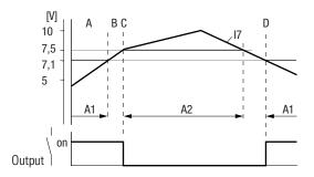
A1 sets relay output Q1 (A) up to a voltage of 7.1V. The hysteresis (B) is between 7.1V and 7.5V. At 7.5V, A2 causes the relay to reset (C). Q1 drops out and does not pick up again until A1 is set at 7.1V (D).
