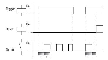
The trigger coil enables the flashing on and off. The flashing period starts with switch position 'off'. The reset coil has priority over the trigger coil and always resets the relay contact.
