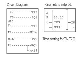
I2 and I3 are converted to one-shot pulses by T6 / T7. Only the actuation of the push-button is recognized. Should they remain constantly pressed, malfunctions would occur. In the above example, T7 does not have to be retentive.
