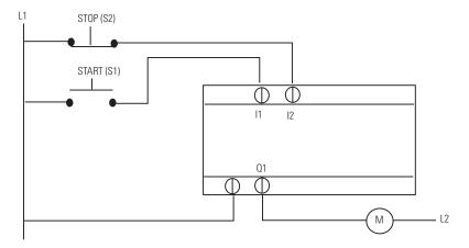
S2 opens the connection to the control voltage in order to turn off the machine. This ensures that the machine will be turned off, even in the event of a wire break.
