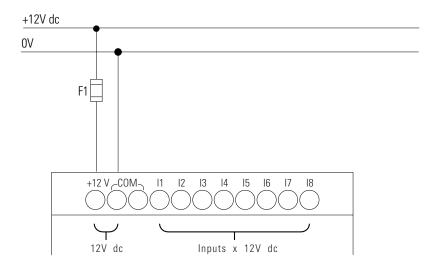
The dc controllers are protected against polarity reversal. To ensure that the unit works correctly, ensure that the polarity of each terminal is correct.
