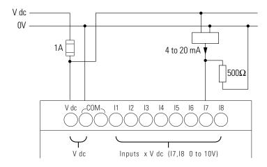
V dc = 12Vdc for 1760-L12DWD V dc = 24V dc for 1760-LxxBWB-xx
