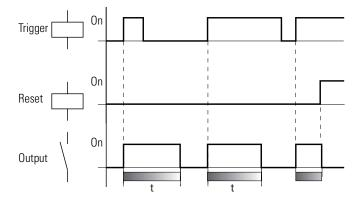
The reset coil has priority over the trigger coil and resets the relay contact before the time has elapsed. If the time is set to zero, the contact is set for the duration of one program scan.
