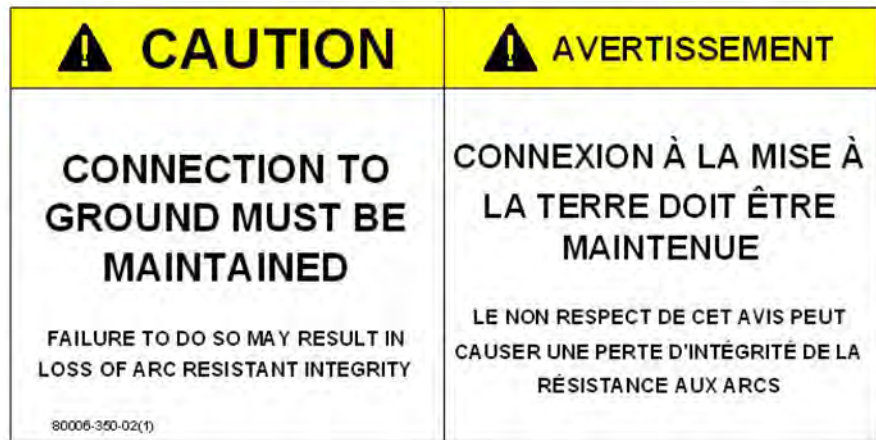
Figure 24 - Side Bus Access Cover Ground Connection (Rear Access Cover)
