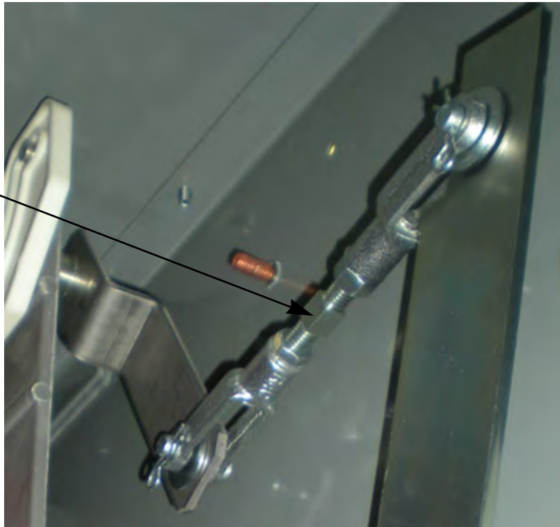
Figure 57 - Isolation Switch Mechanical Threaded Linkage
