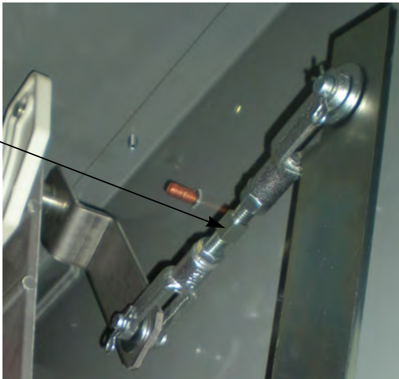
Figure 62 - Isolation Switch Mechanical Threaded Linkage
