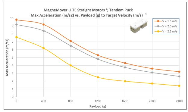
§ Vehicle performance while moving on a straight path. Performance will be reduced when on curves and switches.
