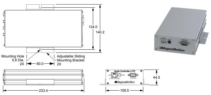
Manages commands and responses from the user's Host Controller to QuickStick<sup>®</sup> or MagneMover<sup>®</sup> LITE Systems. Supports 18 VDC Power Over Ethernet (POE).
