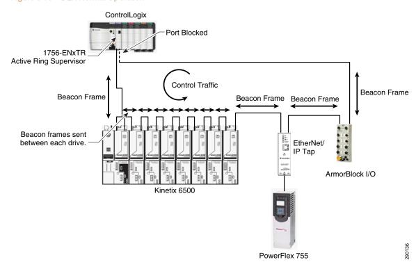
Figure 8-15 DLR Normal Operation
