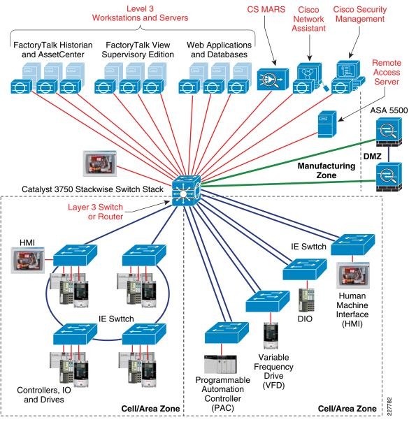
Layer 3 Link – No Switchport, IP Address Assigned
