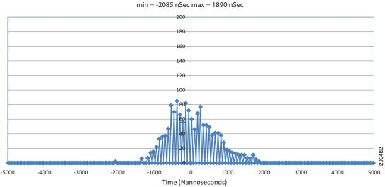
Offset to Master (Nanoseconds) - Reference Drive min = -2085 nSec max = 1890 nSec
