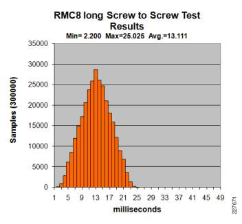
The various test runs of the screw-to-screw tests are summarized in Table 3-14. The table shows that the latency and jitter due to additional industrial Ethernet switches are relatively insignificant compared to the overall IACS network application latency and jitter. The additional latency per-switch hop was approximately 10 µs in the test cases.
