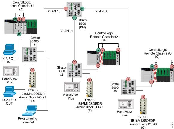
All 1588 PTP devices are connected in a star topology segmented by different VLANS. Each star topology segment is connected to a Stratix 8000 switch, which then connects up to a common 8300 Stratix switch. The Stratix 8000 and 8300 switches are managed switches with full 1588 PTP time synchronization capabilities. These capabilities include transparent, boundary, and forward clock modes. This switch also has QoS and IGMP v2 capabilities, which are enabled by default.
