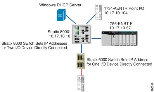
In this example, the Stratix 8000 switch is the DHCP server for both the Rockwell Automation 1756-ENBT and 1734-AENT modules. However, because both the distribution and Stratix 6000 switches act as DCHP servers also tied to the IACS network, multiple DHCP offers could be sent over the subnet. To prevent the 1734-AENT or 1756-ENBT modules from receiving incorrect addresses, DHCP Snooping is enabled on the Stratix 8000 switch.
