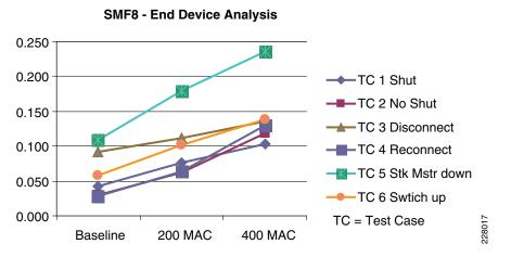
Based on the above graphs, only SMF8 shows a clear trend of increasing network convergence with increasing number of MAC addresses. Based on how STP works and the need to rebuild switching tables (which are MAC-based), there is an expectation that the number of MAC addresses increases the network convergence. The fact that this result is best seen in this test is explained in
