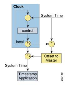
Figure 8-26 Difference Between System Time and Local Time is the Offset to Master
