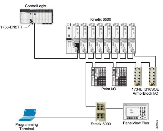
All the non-time-critical components, including the programming terminal and HMI (such as the PanelView Plus) are connected using the Stratix 6000 switch. The Stratix 6000 switch is connected to the end of the linear segment.
