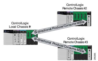
Figure 9-9 Bi-directional Produce/Consume Messaging Traffic Between Controllers
