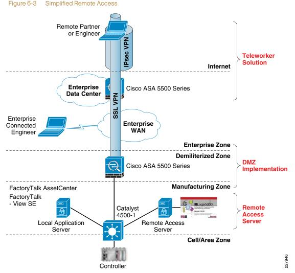
The DMZ is designed to allow sharing data and applications with users or applications not local to the manufacturing environment. A common means would be to replicate critical data onto a server in the DMZ to allow users/applications in the other zone to have visibility to that data. The DMZ is a proxy, allowing other users to make indirect network connections to data and applications residing in other network zones.
