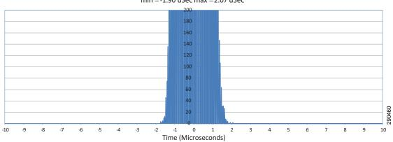
Position Error (Time) - Drive 2 min = -1.90 uSec max = 2.07 uSec
