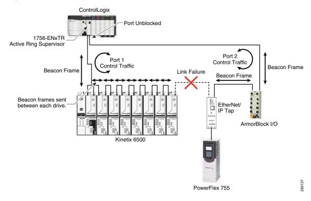
Following detection of the failure, the active ring supervisor begins passing network traffic through both of its ports by unblocking the previously blocked port. Recovery time for a DLR network is typically less than 3 ms for a 50-node network. Note that a DLR can recover only from a single point of failure.
