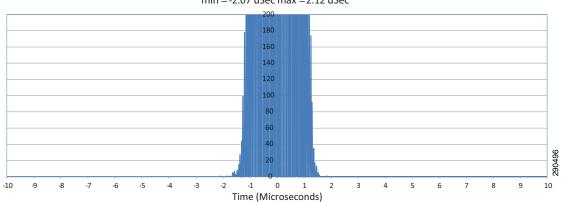
Position Error (Time) - Drive 2 min = -2.07 uSec max = 2.12 uSec
