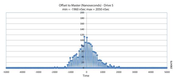
Figure 8-66 Star Architecture Phase Error Test 2.5—Test @ 40% Ixia Traffic Load
