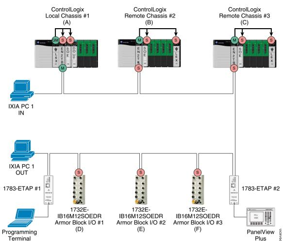
Figure 9-16 shows a diagram of the linear topology.
