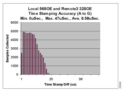
Figure 9-58 Multiple Star Topology—SOE Timestamp Test 3 Results using EN2T Modules with Boundary Clock and Stratix 8000 Switch with Transparent Clock (A to G)
