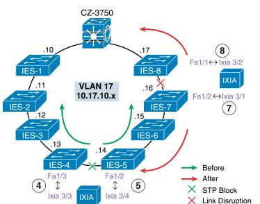
Figure C-1 RMC8—Break Connection Between IES-7 and IES-8
