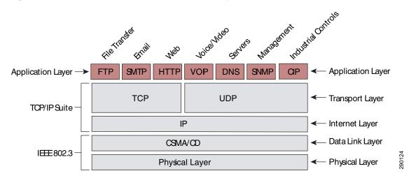
Figure 8-1 CIP Motion Uses Standard Network Stack Implementation
