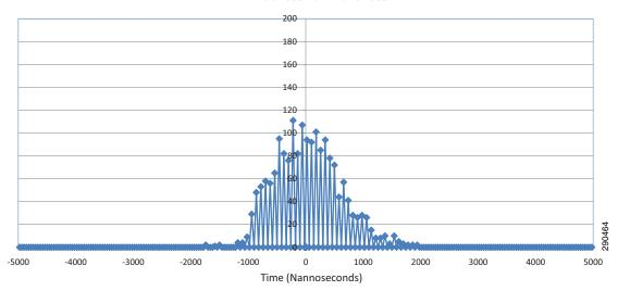
Offset to Master (Nanoseconds) - Reference Drive min = -1790 nSec max = 1910 nSec
