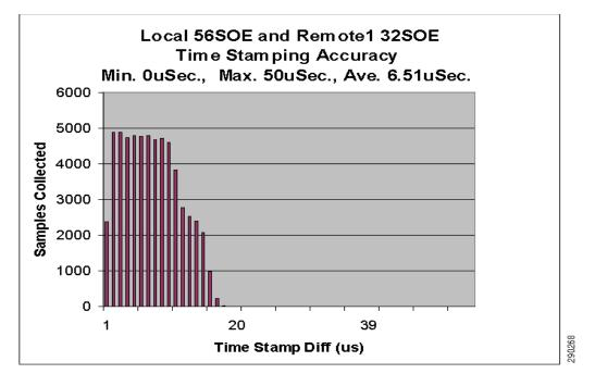
Figure 9-12 Local 1756-IB16ISOE/Remote 1732E-IB16M12ISOEDR Timestamp Difference Test Results
