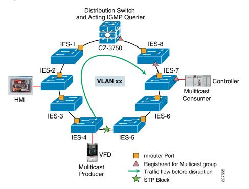
Figure 3-24 depicts a ring topology. Spanning tree is the network resiliency protocol in place. Figure 3-24 shows how the multicast packet traverses the topology from the producer to the consumer. The multicast packet is forwarded in the following manner:
