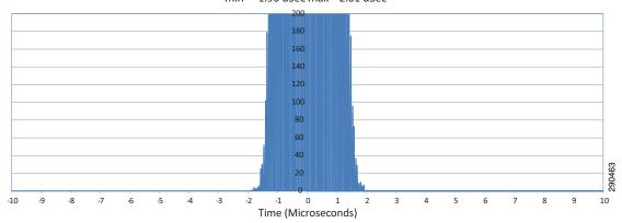
Position Error (Time) - Drive 2 min = -1.96 uSec max = 2.01 uSec
