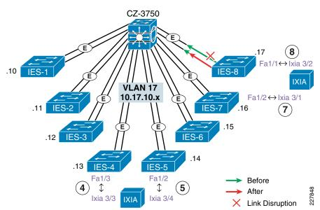
Figure C-7 SEC8—Bring Down Active Link Between IES-8 and 3750
