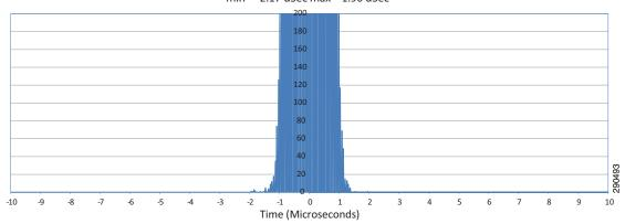
Position Error (Time) - Drive 1 min = -2.17 uSec max = 1.96 uSec
