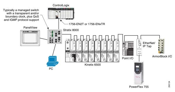
The Stratix 8000 Ethernet switch is shown because a managed switch with a transparent or boundary clock, plus QoS and IGMP protocol support, is typically required in this topology. If an unmanaged switch without these advanced features is inserted in place of the Stratix 8000 switch, time synchronization may not be maintained between master-slaves.
