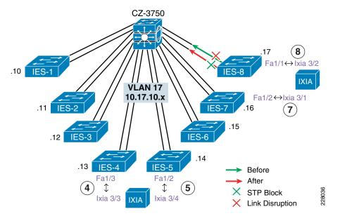
Table C-31 Test Case SMC8-1—Bring Down Active Link Between IES-8 and 3750 (Software)
