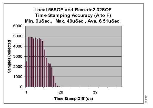
Figure 9-55 Multiple Star Topology—SOE Timestamp Test 3 Results using EN2T Modules with Boundary Clock and Stratix 8000 Switch with Transparent Clock (A to F)
