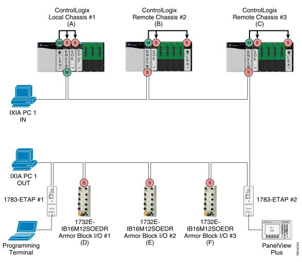
Figure 9-37 Linear Topology Using Embedded Dual-Port Ethernet Switch Devices with Transparent Clock
