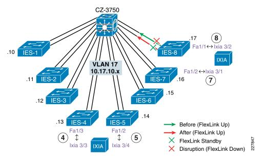
Figure C-10 SFC8—Bring Down Active Link Between IES-8 and 3750
