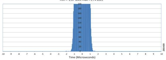
Position Error (Time) - Drive 2 min = -2.07 uSec max = 1.74 uSec
