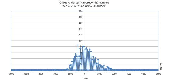
Figure 8-63 Star Architecture Phase Error Test 2.4—Test @ 30% Ixia Traffic Load
