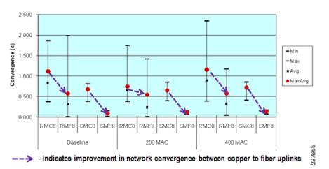
Figure B-7 shows the trend for network convergence after physical cable disconnection (test case 30) copper versus fiber in redundant star topologies with EtherChannel and Flex Link resiliency protocols. The impact of media type is more apparent with copper topologies converging nearly 0.5 seconds slower than fiber topologies.
