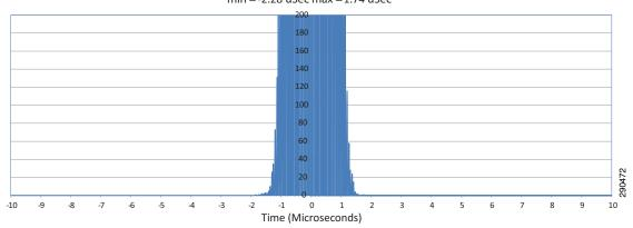
Position Error (Time) - Drive 2 min = -2.28 uSec max = 1.74 uSec
