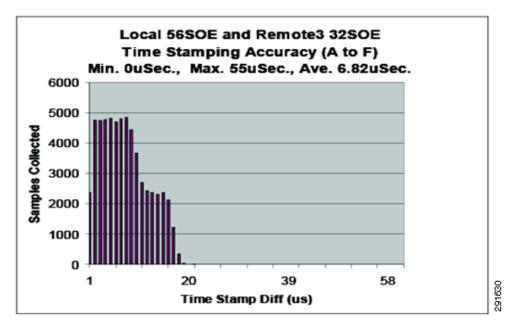
Figure 9-69 Star Topology—SOE Timestamp Test 6 Results Using the Stratix 8300 Switch as Boundary Clock and the Stratix 8000 Switch as Forward Clock (A to F)
