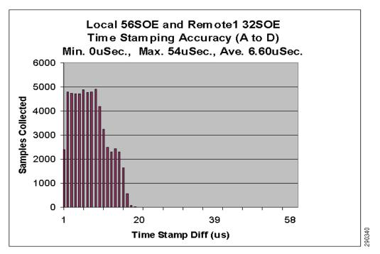
Figure 9-63 Star Topology—SOE Timestamp Test 6 Results Using the Stratix 8300 Switch with Boundary Clock and the Stratix 8000 Switch with Forward Clock (A to D)
