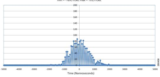
Offset to Master (Nanoseconds) - Reference Drive min = -1895 nSec max = 1935 nSec
