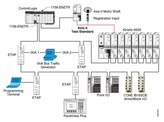
A reference drive (indicated as Axis 0) is used as the reference for all measurements. All measurements, as discussed in Test Criteria, page 8-29, are measured for this architecture.
