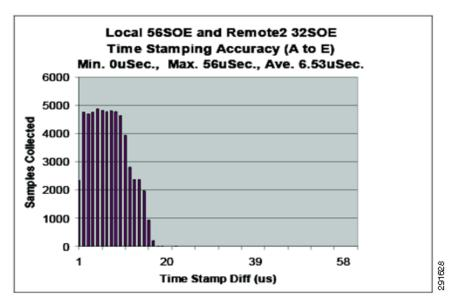
Figure 9-66 Star Topology—SOE Timestamp Test 6 Results Using the Stratix 8300 Switch with Boundary Clock and the Stratix 8000 Switch with Forward Clock (A to E)
