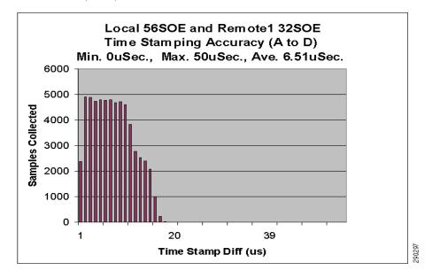
Figure 9-32 Star Topology—SOE Timestamp Test 3 Results Using the Stratix 8000 with Transparent Clock (A to D)
