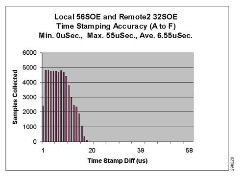
Figure 9-56 Multiple Star Topology—SOE Timestamp Test 6 Results using 1756-EN2T Modules with Boundary Clock and Stratix 8000 Switches with Forward Clock (A to F)
