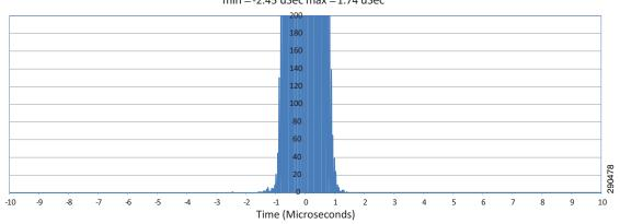
Position Error (Time) - Drive 4 min = -2.45 uSec max = 1.74 uSec
