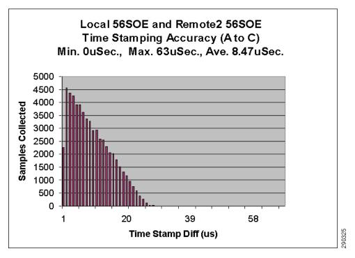
Figure 9-47 Multiple Star Topology—SOE Timestamp Test 6 Results using 1756-EN2T Modules with Boundary Clock and Stratix 8000 Switches with Forward Clock (A to C)
