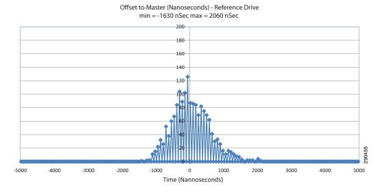
Figure 8-45 Linear Architecture Phase Error Test 1.4—Test @ 30% Ixia Traffic Load
