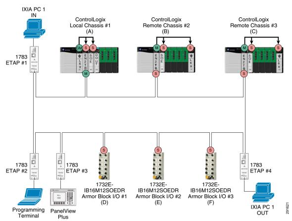
Figure 9-17 shows a diagram of the ring topology.
