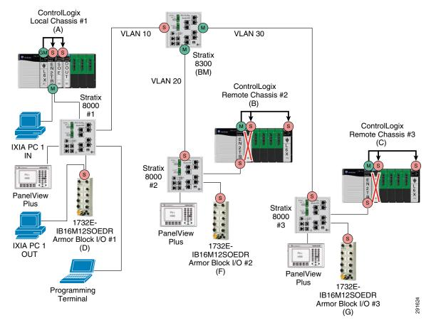
The test configuration seen in Figure 9-60 could not be conducted because the 1756-IB16ISOE module does not support a unicast connection at this time. This has been illustrated with a red X over the remote 1756-IB16ISOE modules. Instead, a simpler test was conducted with the local 1756-IB16ISOE and remote 1756-IB32SOE modules. This test was successful.
