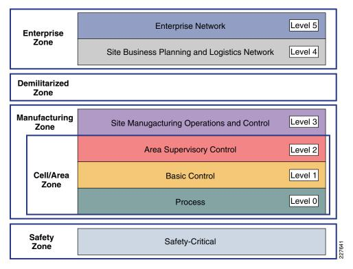
This model identifies levels of operations and defines each level. In this *DIG, levels* refer to this concept of levels of operations. The Open Systems Interconnection (OSI) and Reference Model is also commonly referred to when discussing network architectures. The OSI model refers to layers of network communication functions. In this *DIG*, unless specified, *layers* refer to layers of the OSI model.
