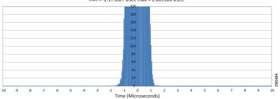
Position Error (Time) - Drive 6 min = -2.179827 uSec max = 1.689366 uSec
