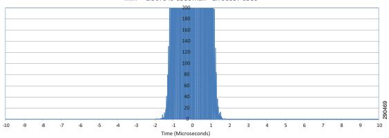
Position Error (Time) - Drive 2 min = -1.907349 uSec max = 1.798357 uSec
