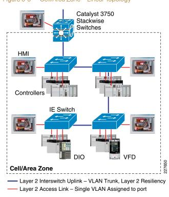
Figure 3-6 Cell/Area Zone—Linear Topology
