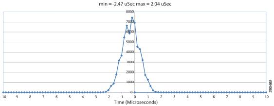
Phase Error (Time) min = -2.47 uSec max = 2.04 uSec
