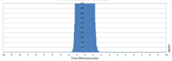
Position Error (Time) - Drive 2 min = -2.01 uSec max = 2.07 uSec
