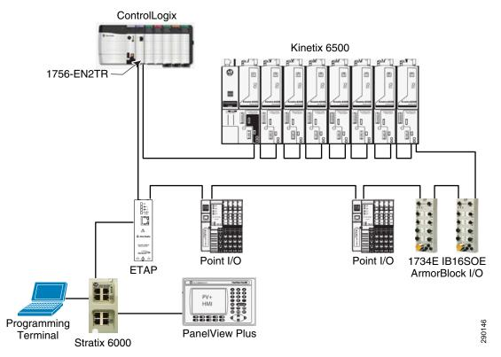
A DLR or ring topology has a distinct advantage over a linear topology. Because of the closed loop nature of a DLR, it is resilient to a single point of failure on the network. That is, if a link is broken in the DLR, the ring can recover from a single fault and maintain communications. This failure point can occur anywhere on the ring, even between daisy-chained (Kinetix 6500) drives, and the DLR is still able to recover fast enough to avoid application disruption.
