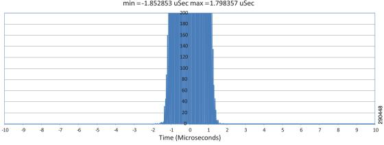
Position Error (Time) - Drive 2 min =-1.852853 uSec max =1.798357 uSec
