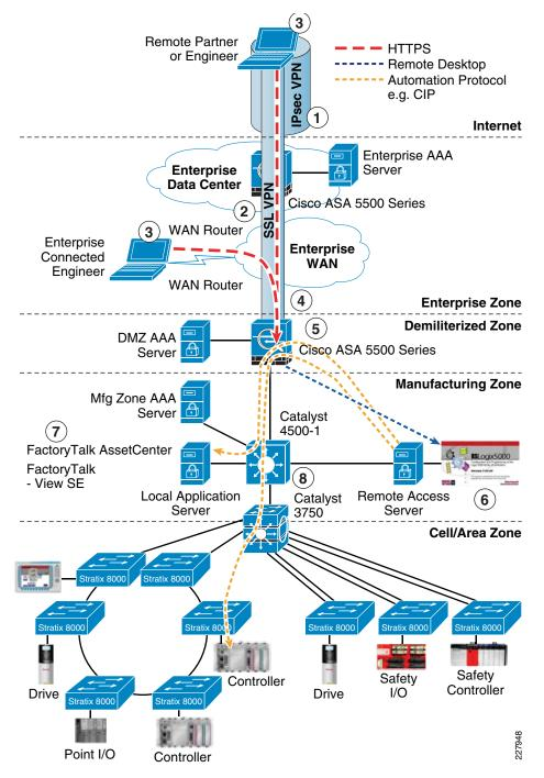
Figure 6-5 Detailed View of Remote Access to Industrial Automation and Control Systems
