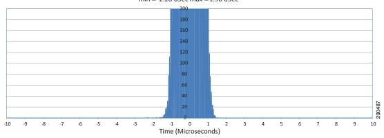
Position Error (Time) - Drive 6 min = -2.28 uSec max = 1.96 uSec
