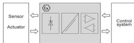
Figure 1 - Function – Isolating, Amplifying and Transforming Signals
