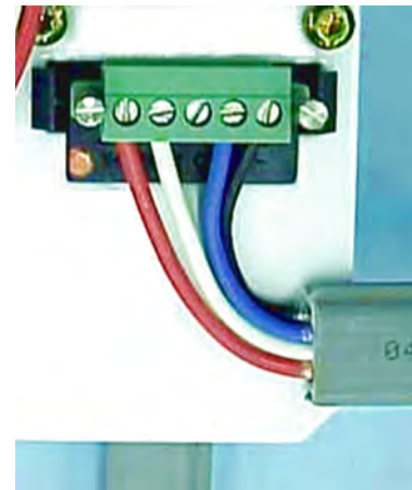
Front View of DeviceNet Splice (Series M)
