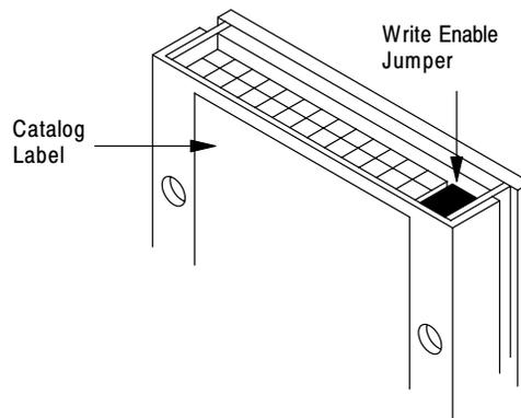
To remove or insert the write enable jumper into the EEPROM module use a pair of needle nose pliers.
