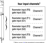
Each gate input has a corresponding gate jumper. You can set each gate jumper for +5-12V or +12-40V operation.
