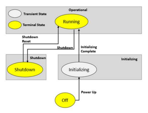
Axes with the Test Mode attribute set to Enabled and that are configured for Controller Loop Back simulate these transitions for the Axis State Model of a Feedback Only axis or CIP Motion Encoder.
