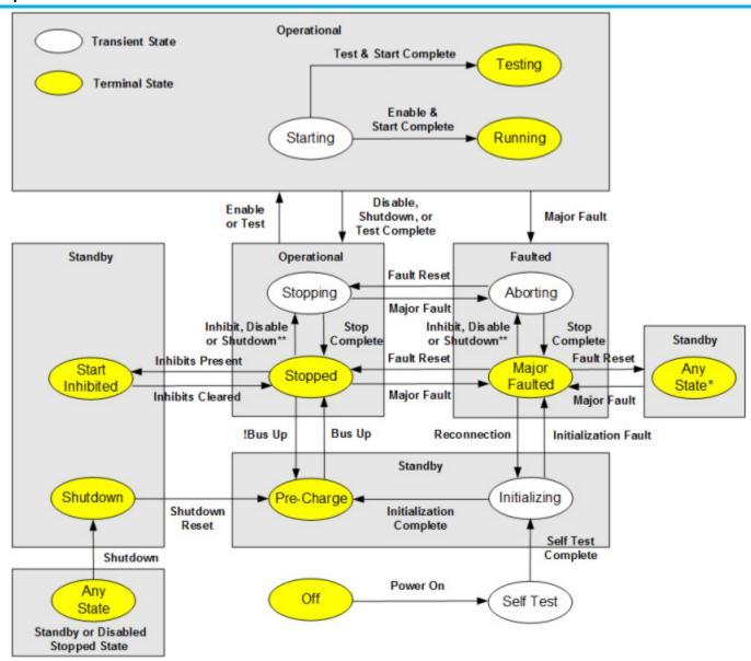
**Tip:** \* Specific Standby State after a Fault Reset is determined by applying the Fault Reset State Transition Precedence Rules.
