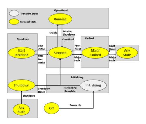
Axes with the Test Mode attribute set to Enabled and that are configured for Controller Loop Back simulate these transitions for the Axis State Model.
