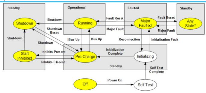
**Tip:** \*Specific Standby state after a fault reset is determined by applying Fault Reset State Transition Precedence rules.
