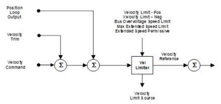
Through these extensions to the Velocity Limiter function, a drive that supports field weakening can be configured to manage extended speed operation, only allowing operation above  $S_{\rm OV}$  by setting the PM Motor Extended Speed Permissive attribute. Systems that can run safely above  $S_{\rm OV}$  are equipped with a DC Bus Regulator or a Resistive Brake Module.
