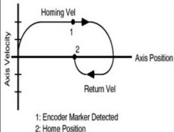
The accuracy of this homing sequence depends only on the time delay in detecting the marker transition. The position uncertainty of the home position is the product of the maximum delay for the control to detect the marker pulse (~1 microsecond) and the specified Home Speed.
