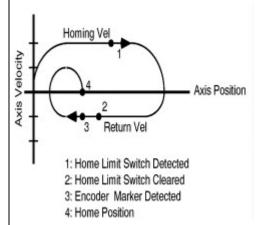
If the controller detects that the state of the home switch at the start of the homing sequence is active, the controller immediately reverses the homing direction and begins the return leg of the homing sequence.
