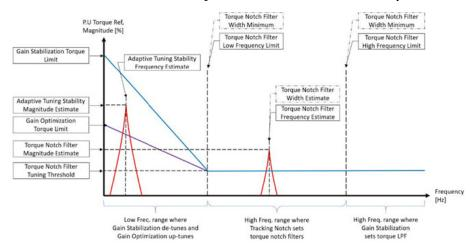
When a low frequency resonance is detected with an Adaptive Tuning Stability Magnitude Estimate less than the Gain Optimization Torque Limit threshold line (purple), Gain Optimization increases the Adaptive Tuning Gain Scaling Factor to greater than 1.0 in additive increments until the low frequency resonance magnitude increases above this threshold line. This additive increment is fixed and equal to the Gain Optimization Scale
