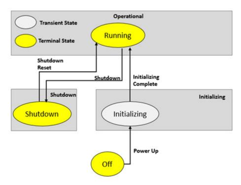
Axes with the Test Mode attribute set to Enabled and that are configured for Controller Loop Back simulate these transitions of a CIP Motion Non-regenerative Converter axis.
