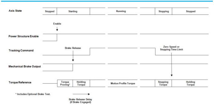
**Tip:** Recommended criteria for Zero Speed is based on Velocity Feedback, or in the case of Frequency Control drive, based on Velocity Reference. Zero Speed criteria can be established explicitly through optional Zero Speed and Zero Speed Time attributes or implicitly as 1% of motor rated speed or left to the drive vendor's discretion.
