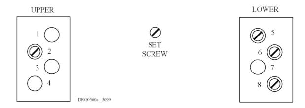
Figure 2-1 Chassis mechanical coding block configurations
