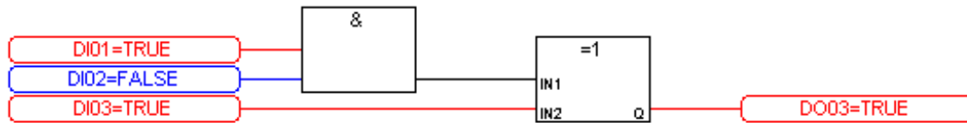
Figure 48 Power Flow Debugging Off
