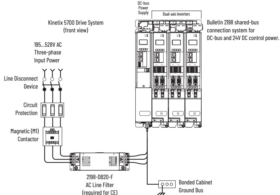
**IMPORTANT** Axis motoring and regeneration power requirement determines the size of the DC-bus power supply, and the shunt and capacitance requirement. See Motion Analyzer for sizing your Kinetix 5700 application.
