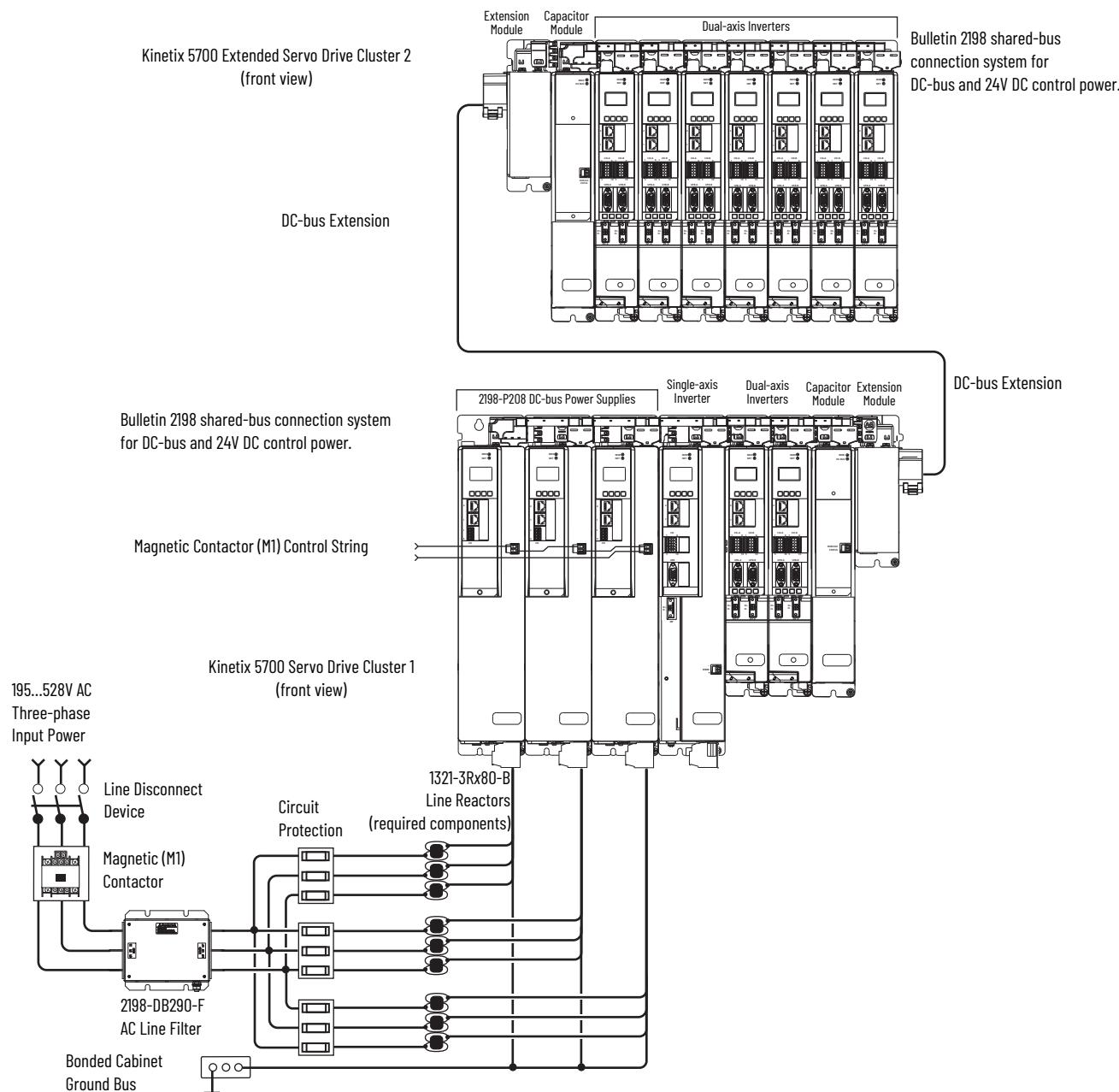
**IMPORTANT** When two or three DC-bus power supplies are wired together in the same drive cluster, they must all be catalog number 2198-P208.
