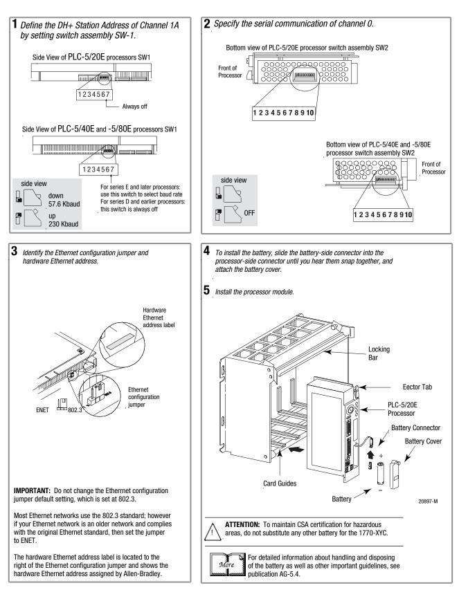
Install the PLC-5 Processor
