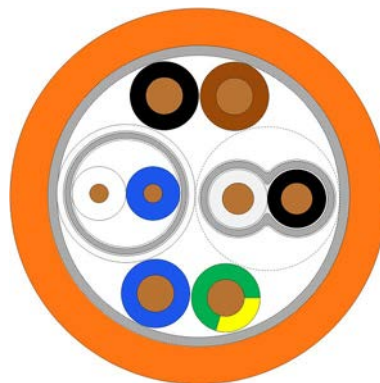
2090-CSBM1xx-xxLFxx and 2090-CSxM1xx-xxVAxx Cables Cross-sectional View
