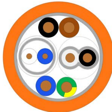
2090-CSBM1xx-xxLFxx and 2090-CSxM1xx-xxVAxx Cables Cross-sectional View
