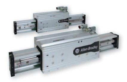
To produce a high-speed, load-bearing linear actuator today, many machine builders invest a lot of time and money to design a mechanism with rotary-to-linear motion conversion. With the Allen-Bradley Integrated Linear Thruster, machine builders can get high-speed, load-bearing linear motion out-of-the-box. The LDAT-Series Integrated Linear Thruster is a reliable, high-speed linear actuator with an integrated linear guide that is capable of pushing, pulling or carrying a load.
