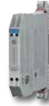
The diode return feature prevents a current into the hazardous area, therefore the current assumption for intrinsic safety calculations is zero
