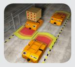
In AGV applications, two warning fields can gradually slow the AGV thus reducing brake wear.
