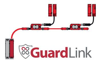
The interlock or E-Stop is connected to a GuardLink enabled connection tap that features local safety diagnostics in a trunk and drop topology. The taps are connected together in a series using standard 4-wire cables with M12 connectors. The linked system is then interfaced to the Guardmaster DG Dual GuardLink safety relay and to the Connected Enterprise via the 440R-ENETR EtherNet/IP interface.
