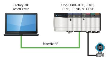
FDT Technology standardizes the communication interface between field devices and host systems to reduce integration efforts. FactoryTalk AssetCentre Process Device Configuration is enabled by FDT Technology.
