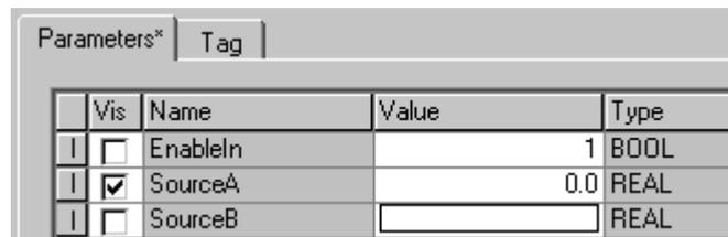
2. On the **Parameters** tab, in the **Value** box of the desired parameter, type the value.
