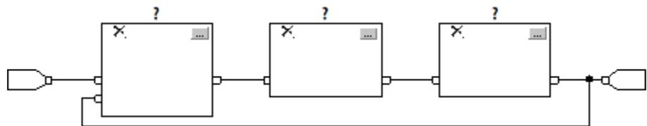
To identify which block to execute first, mark the input wire that creates the loop (the feedback wire) with the **Assume Data Available** indicator. In this example, block 1 uses the output from block 3 that was produced in the previous execution of the routine.
