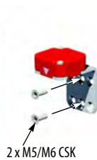
For proper installation, a minimum of two fasteners must be used, at least one of which must be fitted to the top row of holes, closest to the bend in the actuator mounting bracket.
