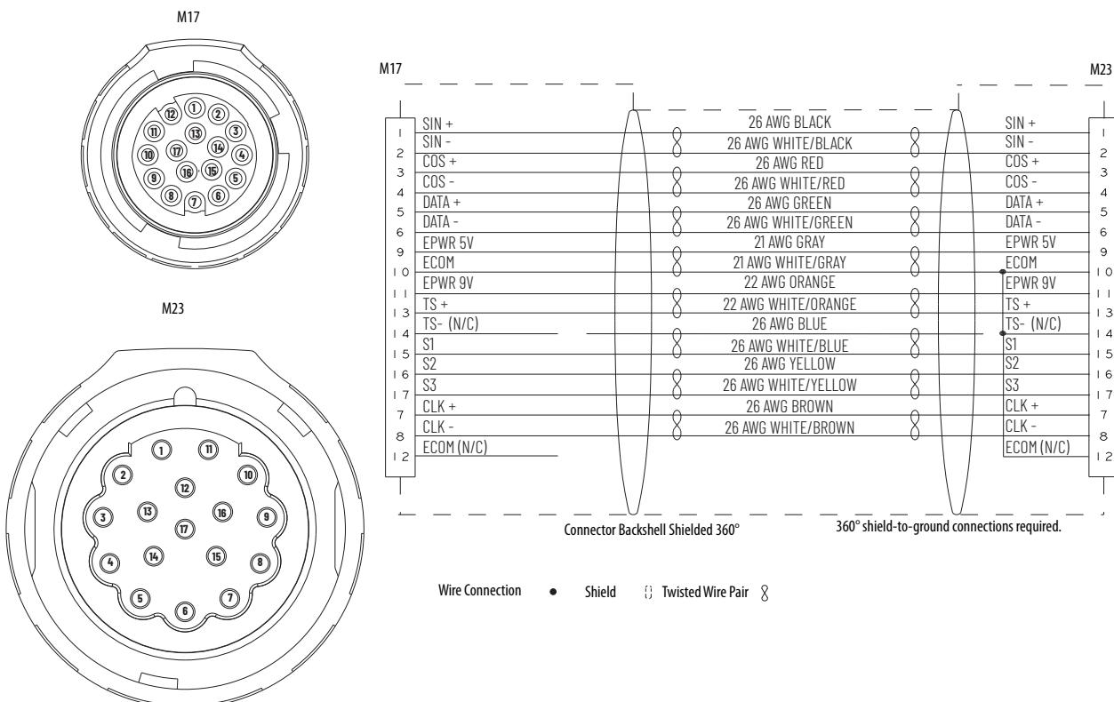
**DSD Auxiliary Feedback Cable (2090-CFBFLS7-CDAFx)**
