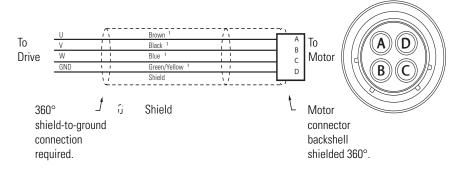
1 Wire gauge (8 AWG) and connector keying is based on motor power requirements. Refer to Kinetix Motion Control Selection Guide, publication <u>GMC-SG001</u>, for additional information.
