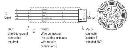
1 Wire gauge (10, 12, 14, or 16 AWG) and connector keying varies based on motor and power requirements. Refer to Kinetix Motion Control Selection Guide, publication <u>GMC-SG001</u>, for additional information.
