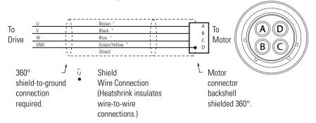
1 Wire gauge (10, 14, or 16 AWG) and connector keying varies based on motor and power requirements. Refer to Kinetix Motion Control Selection Guide, publication <u>GMC-SG001</u>, for additional information.
