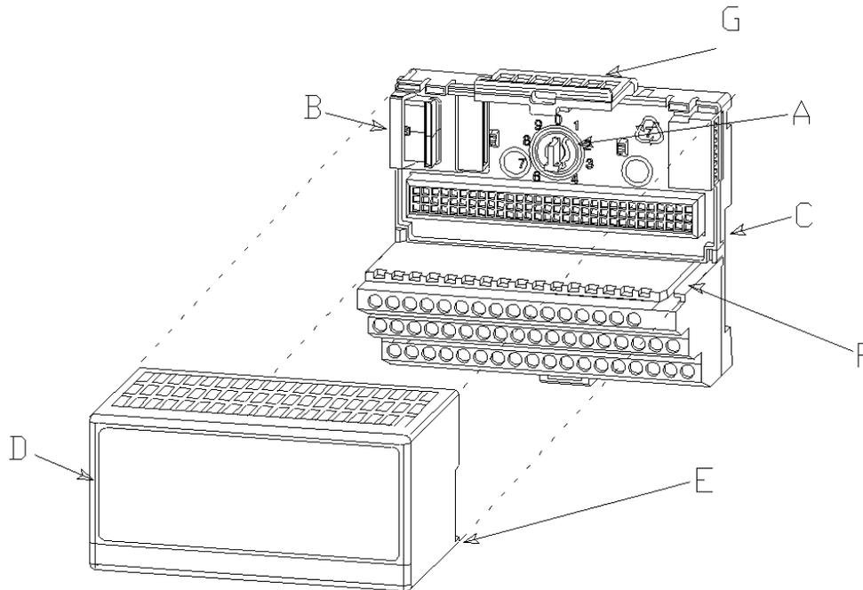
2. Verify the side connector (B) is pushed fully to the left.
