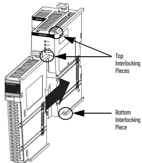
7. Verify that the module is installed in one of the following ways:
