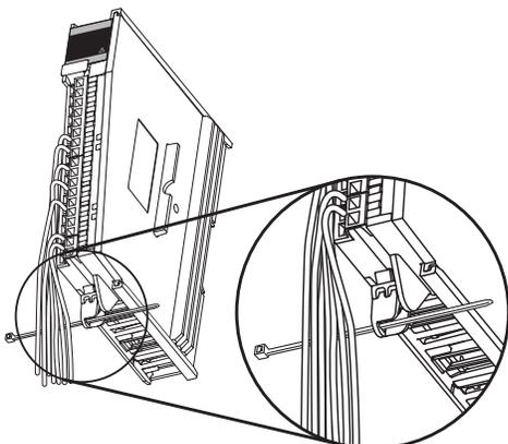
4. Wrap the cable tie around the wires and secure it.
