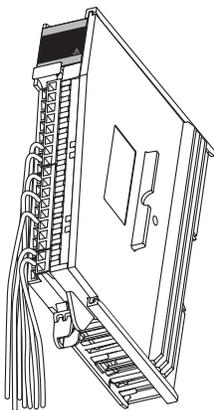
3. Thread the cable tie through the lower hook at the bottom of the RTB.
