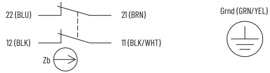
Figure 2 - Contact Opening Characteristics
