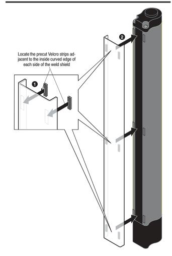
Note: Each weld shield kit comes with a total of 24 Velcro strips. GuardShield's with smaller protective heights may not require the attachment of all strips. Use your discretion in the number of strips applied.
