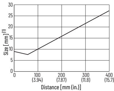
Figure 5 - Background Suppression (400 mm Spot Size)
