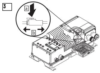
Connect the Cable of the Replacement Fan
