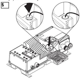
Replace the Fan using the Fan Guard from Step  $\underline{\mathbf{3}}$  , and Tighten the Screws
