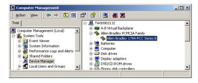
Double-click Allen-Bradley 1784-PCC Series B to bring up its Properties screen. Select the Driver tab.
