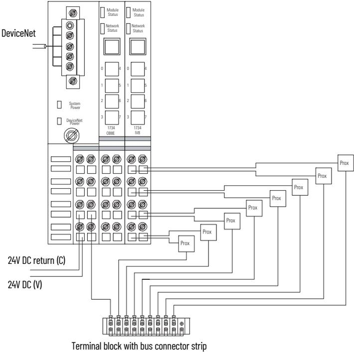
Figure 6 - Wiring Example of 1734-IV8, 1734-IV8K Using 3-Wire Proximity Switches
