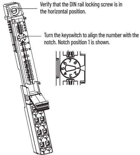
3. Insert the module straight down into the mounting base and press to secure. The module locks into place.
