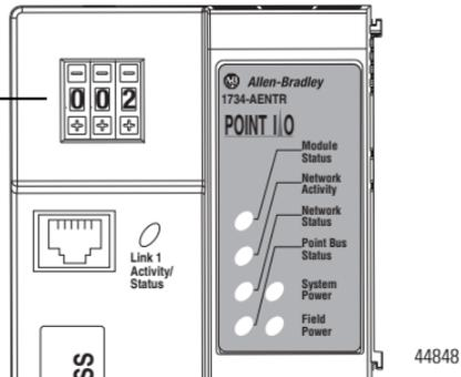
If you set the switches to an invalid number (for example, 000 or a value greater than 254 excluding 888), the adapter checks to see if you enabled DHCP.
