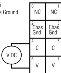
**IMPORTANT** Do not connect 120/240V AC power to this supply. This DC supply will be connected to the internal power bus.
