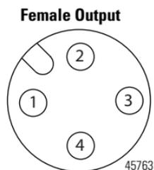
The power required by the module is based on a 4-pin micro-style connector system. Power can be daisy chained through the module either left to right or right to left. The standard configuration is with Module/Auxiliary power entering the module on the left connector.
