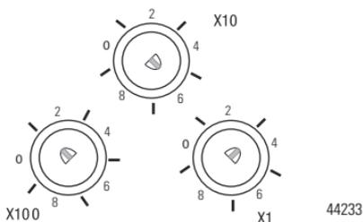
When the switches are set to a valid number, the I/O block's IP address is 192.168.1.xxx, where xxx represents the number set on the switches. The I/O block's subnet mask is 255.255.255.0 and default gateway address is set to 192.168.1.1.
