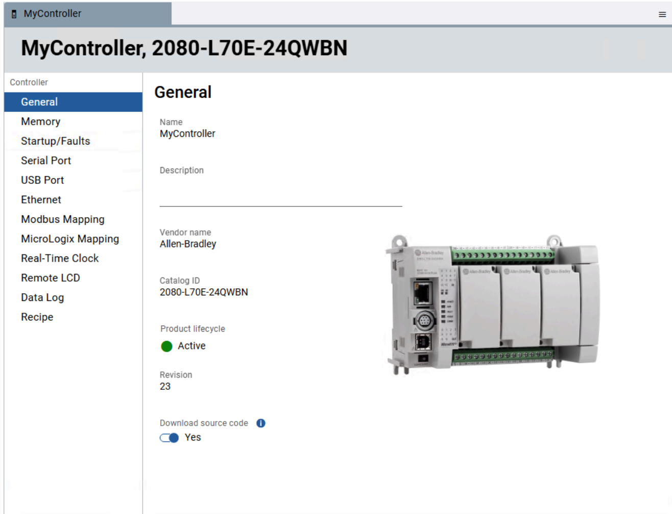
Figure 8. Controller tree and the General configuration page of an Micro870 L70E controller
