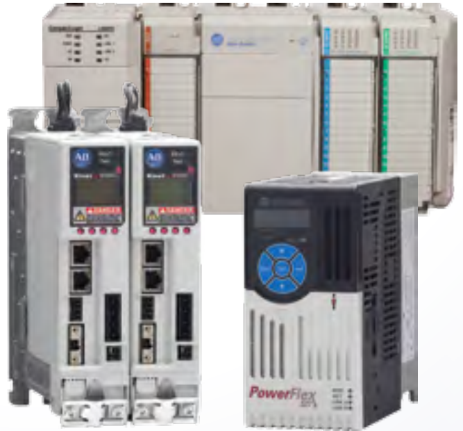
For applications that require both simple speed control as well as precise motor functionality, a combination of AC and servo drives is the logical solution. The PowerFlex 527 AC drive manages the simple speed control while a Kinetix servo drive handles the more precise motor control operations involving speed, torque and position control.
