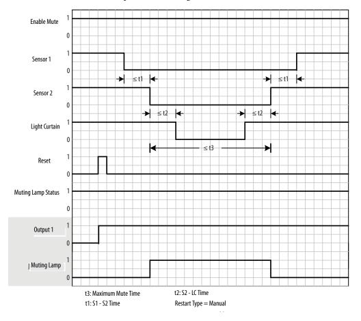
The diagram provides a visual illustration of the operation of the light curtain.
