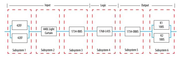
Calculations are based on one operation of the light curtain per hour, or 8,760 operations of the contactors per year.
